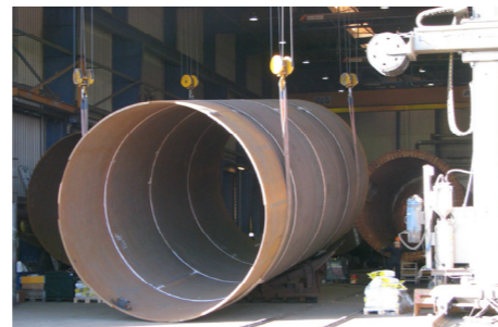
Monopile production in Aalborg
